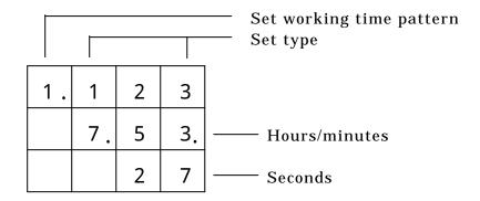
If the power is turned on within the working time, the screen advances to the following reference screen in a few seconds. If the power is turned on before the working time starts, the screen advances to the reference screen whenever the working time starts or the actual results are input.
