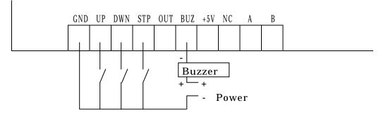
For the no-voltage contact point to be connected to the count(UP,DOWN,STP), a stable 5V voltage and 10mA current which can be turned on and off should be used. There should be a minimum of chattering.
